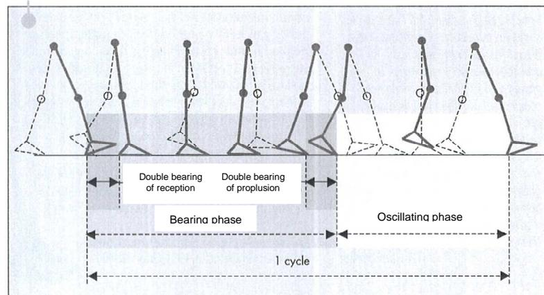
Fig. 2. Diagrammatic representation of the walking cycle and its main phases and sub-phases [6].
