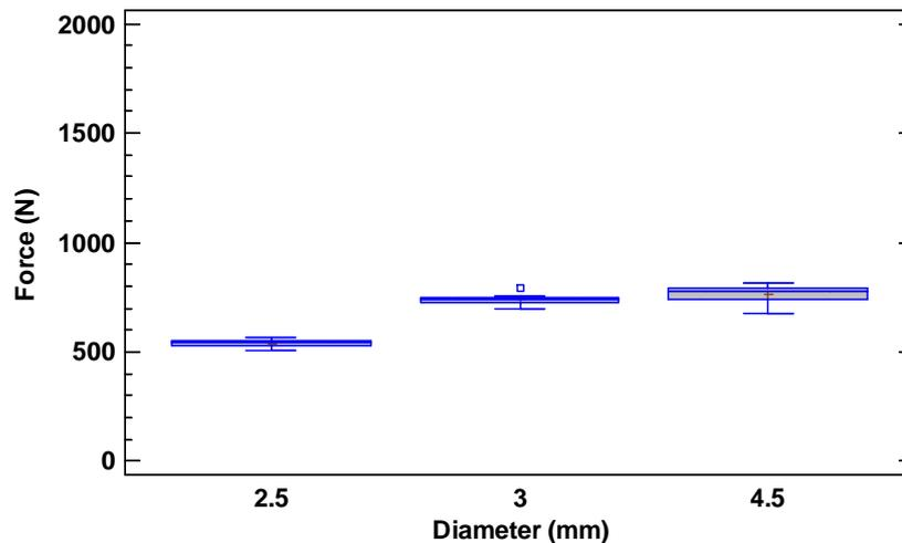
Fig. 16. Perforation forces as a function of nail diameter, pyramidal tip, a truncation of 1 mm and an angle of 30°.
