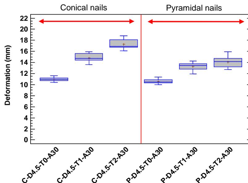
Fig. 14. Insert deformations as a function of nails with different shapes and truncations.
