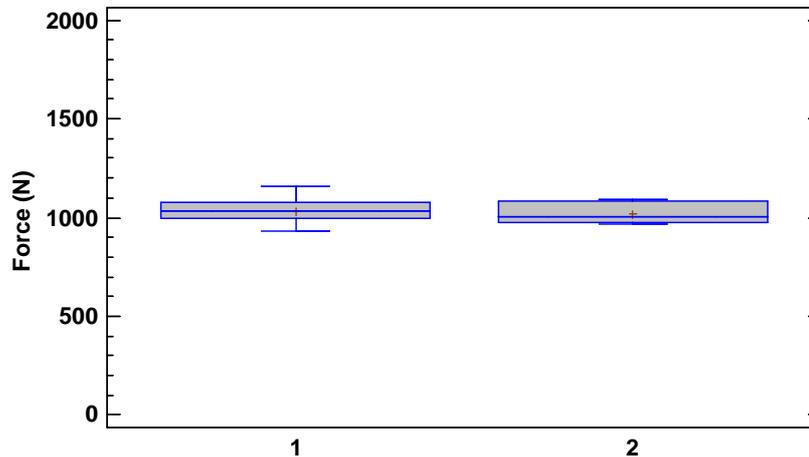
Fig. 10. Perforation forces for two standardized nails C-D4.5-T1-A30.
