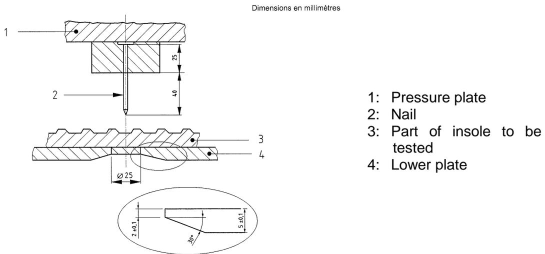
Fig. 22. Device used for the perforation resistance test.
