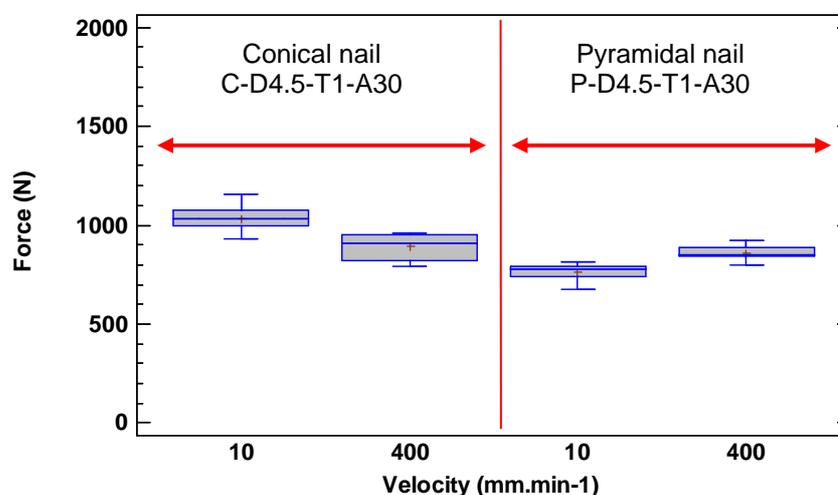
Fig. 17. Perforation forces for two different penetration velocities.
