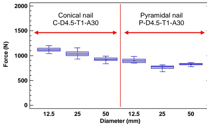
Fig. 18. Perforation forces for different sample clamping platen hole diameters.
