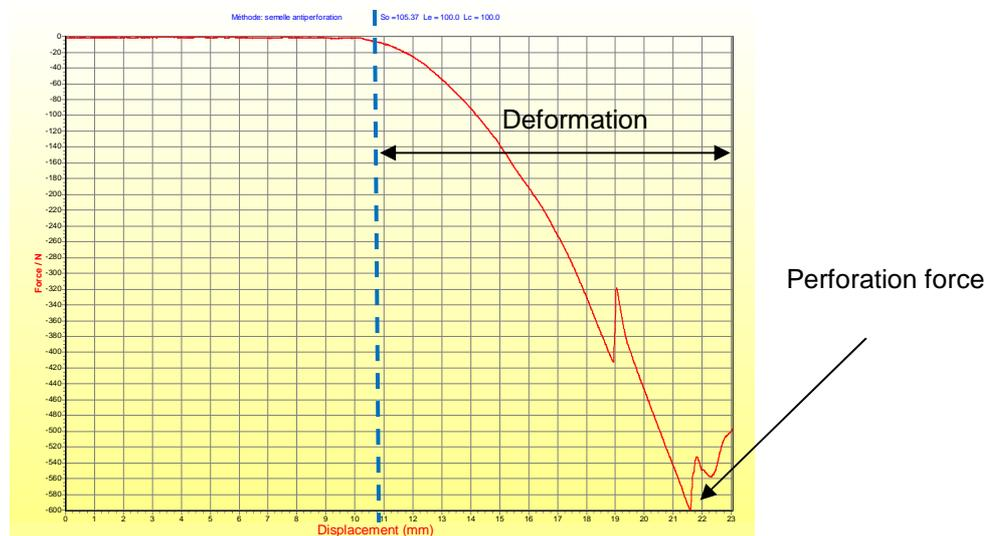
Fig. 6. Example of the curve of nail displacement as a function of force applied on the textile insert.
