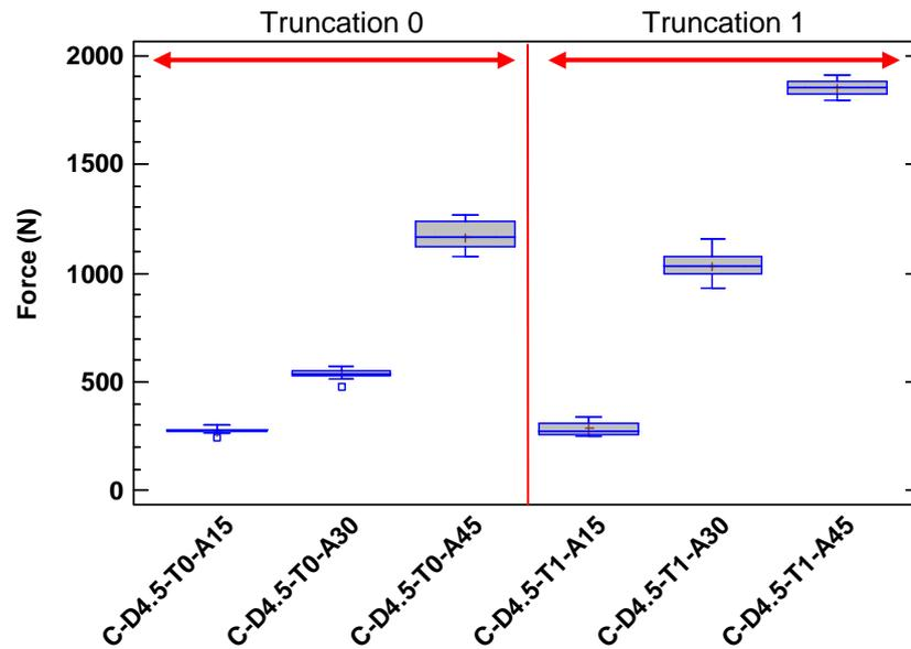
Fig. 13. Perforation forces as a function of different tip angles and truncations.
