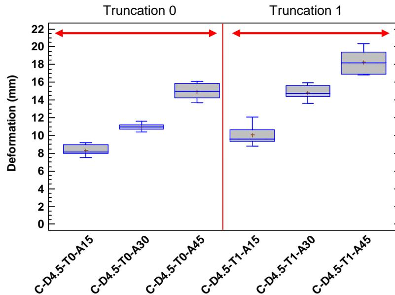
Fig. 15. Deformations of the insert as a function of different nail angles and truncations.
