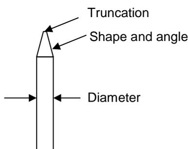
Fig. 7. Nail characteristics.
