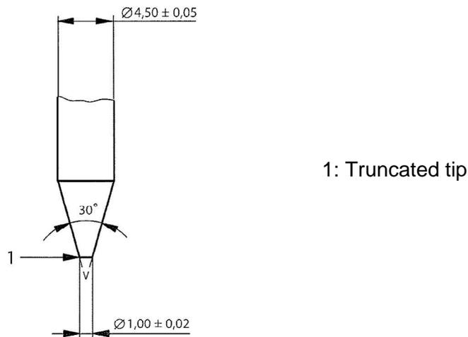
Fig. 23. Standard nail for the perforation resistance test.
