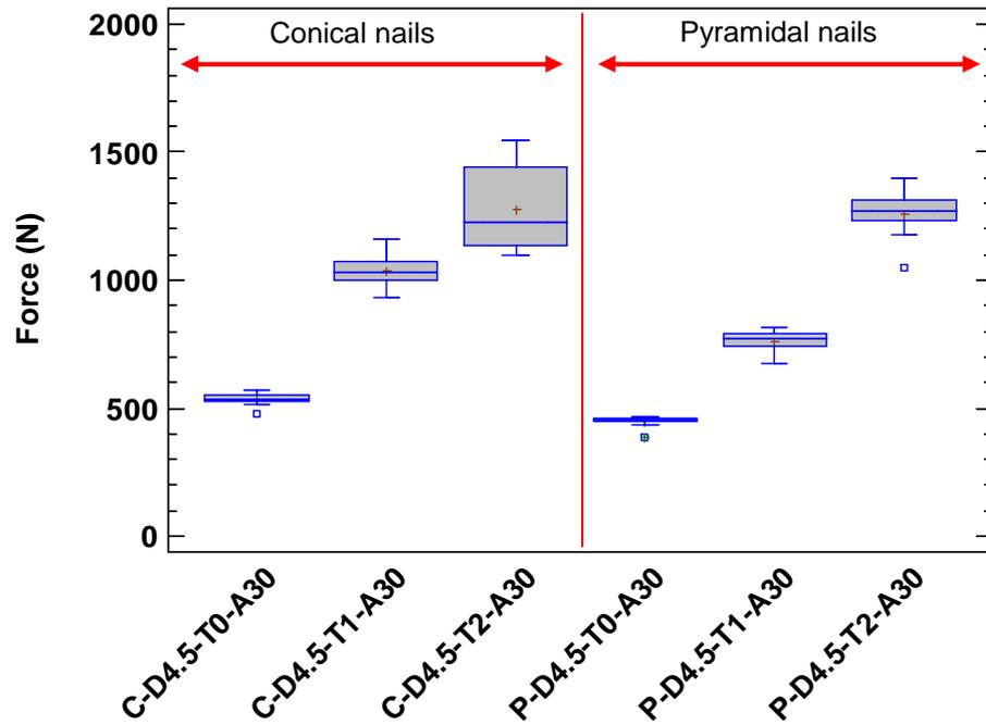
Fig. 12. Perforation forces as a function of nails with different shapes and truncations.
