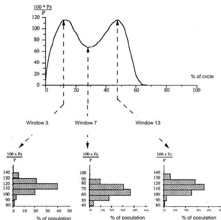
Fig. 3.  $F_z/P$  ratio curves (vertical reaction/weight) as a function of the walking cycle and distributions for windows 3, 7 and 13 [7].
