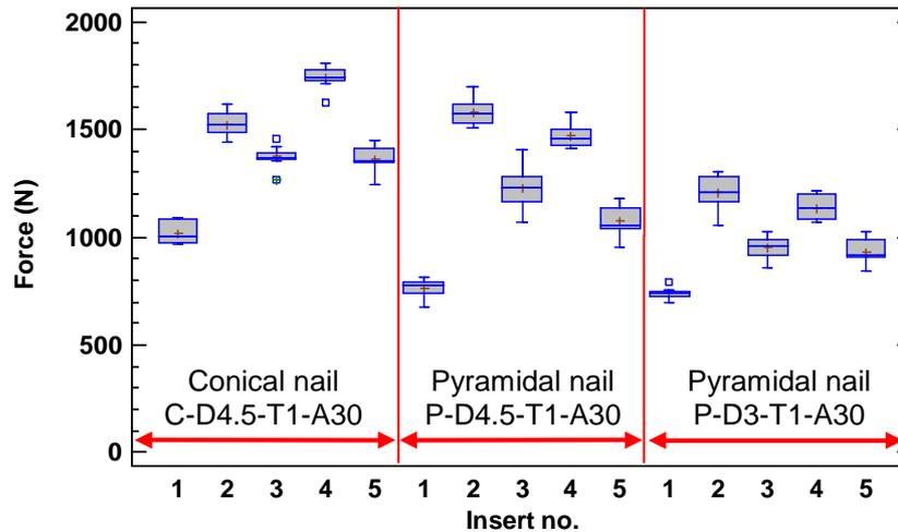
Fig. 20. Perforation forces as a function of insert quality.
