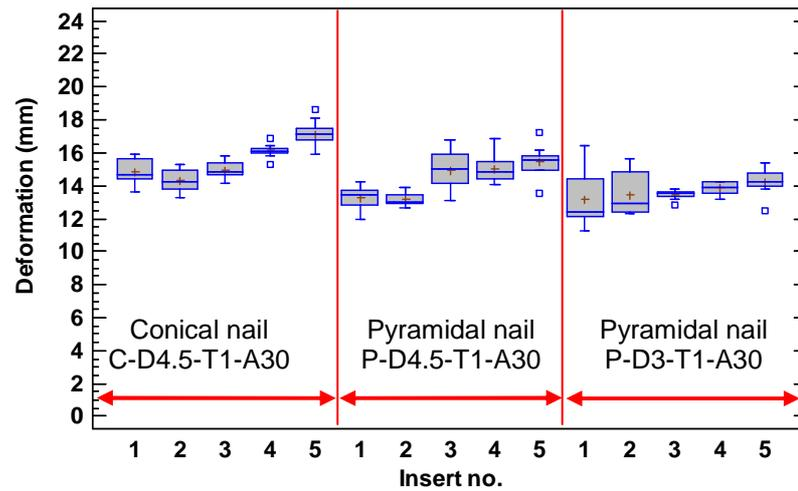
Fig. 21. Deformations as a function of insert quality.
