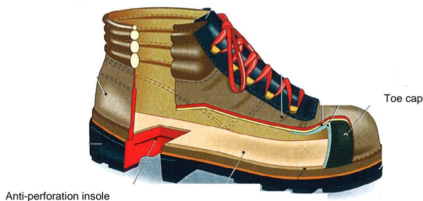
Fig. 1. The different components of a safety shoe.
