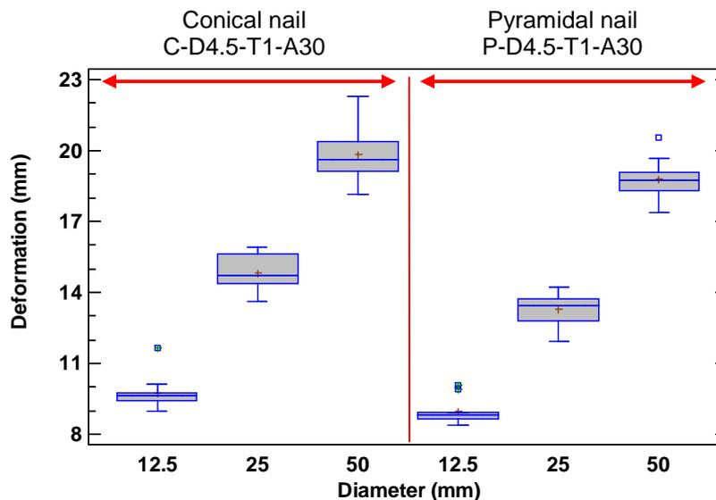
Fig. 19. Deformations as a function of the sample clamping platen hole diameters.
