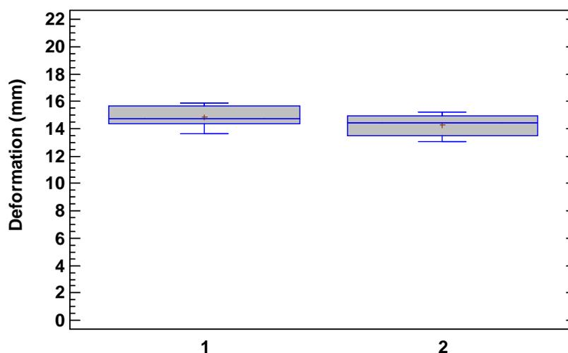
Fig. 11. Deformations of the insert for two standardized nails C-D4.5-T1-A30.
