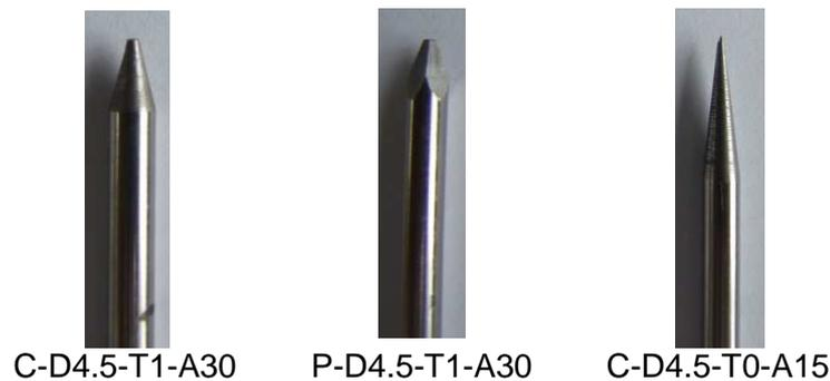
Fig. 8. Examples of nails with different geometries.
